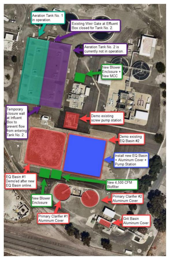
A schematic of the new EQ basins and pump station geometry is provided below:
