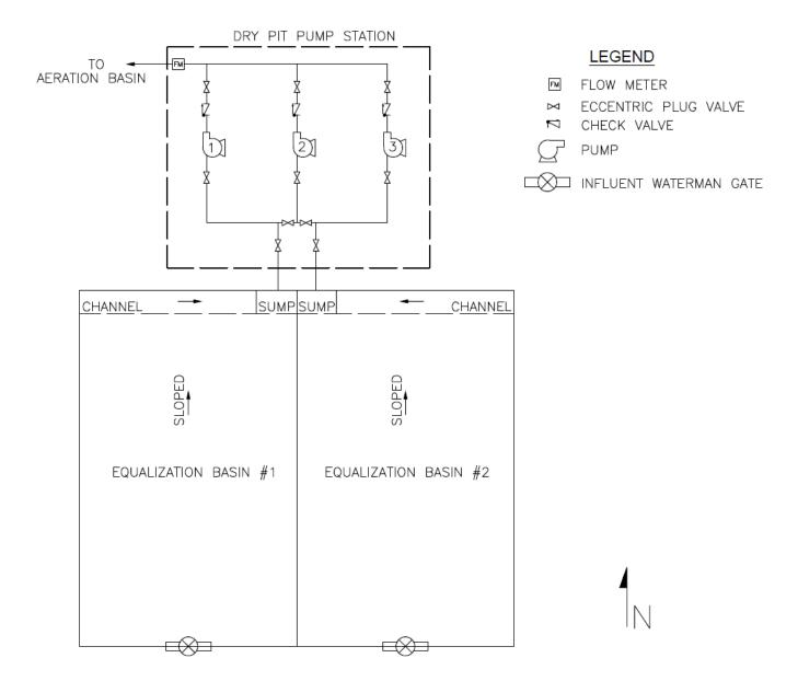
Flow equalization system design parameters are:
