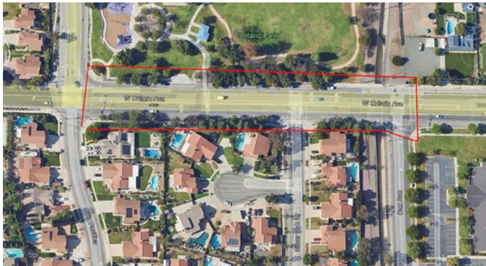
Figure 2: Portion of W. Ontario Avenue between Oak Avenue and Via Pacifica. Improvements include grind and overlay, and possibly sidewalk and/or access improvement at the intersections.
